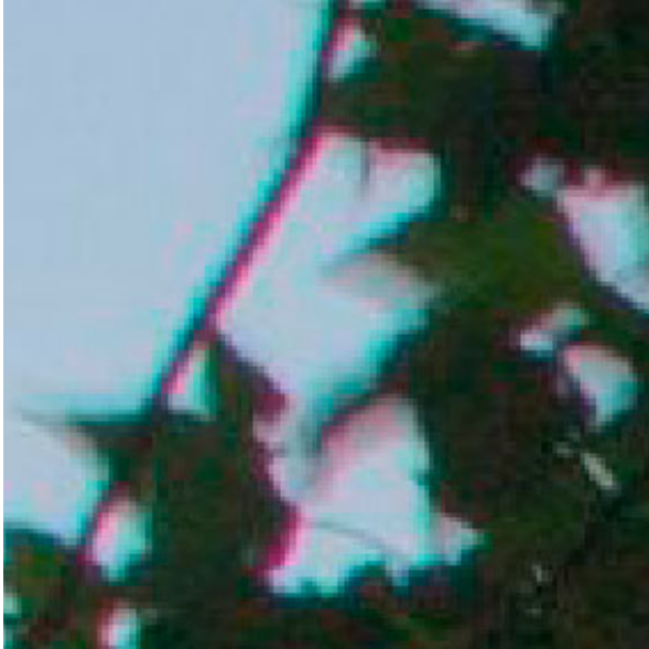
Chromatic aberration produces the classic green-purple fringe (enlarged 235%)
